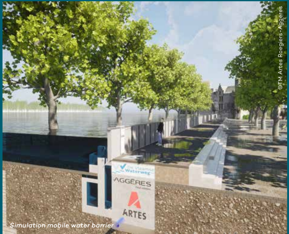
Water barrier integrated in the quay plain
